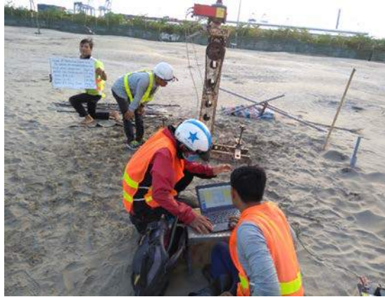
Field vane shear test after ground improvement
