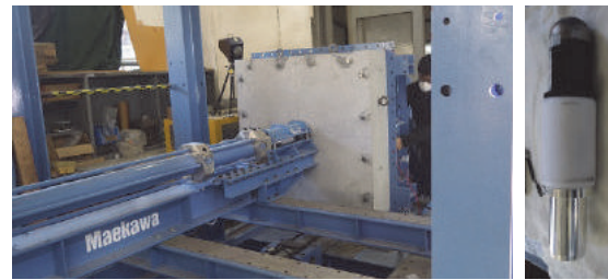
Figure 2: Experiment setup (left: launch device, right: projectile)
